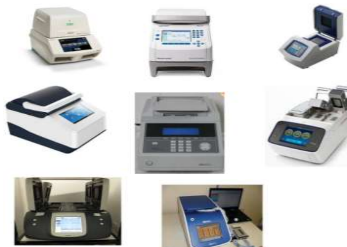
Figure 3. Showing various types of Polymerase chain reaction (PCR). Polymerase chain reaction PCR method. PCR is a very sensitive technique that allows rapid amplification of a specific segment of DNA. PCR makes billions of copies of a specific DNA fragment or gene, which allows detection and identification of gene sequences using visual techniques based on size and charge. Source: https://www.thermofisher.com/us/en/home/life-science/cloning/pcr-amplification/pcr-basics/what-is-pcr.html
