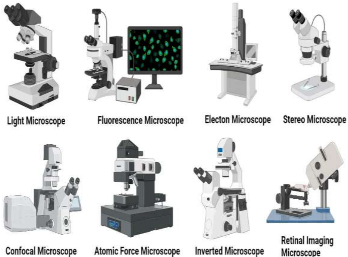
Figure 1. Some common microbiological technology devices (Some images of various microscopes types) used. A microscope is an instrument that is used to magnify small objects. Microscopes opened a window into the invisible world of microorganisms. Some microscopes can even be used to observe an object at the cellular level, allowing scientists to see the shape of a cell, its nucleus, mitochondria, and other organelles. Source: https://thebiologynotes.com/types-of-microscopes/#2-compound-microscope
